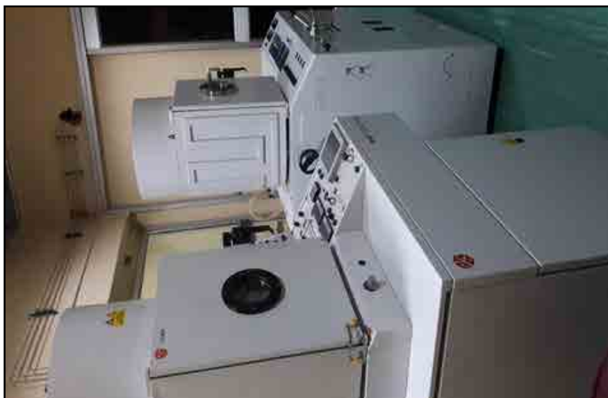
2. Vacuum evaporation and deposition systems (FL 300 and BC 300) from Hind High vac, Bangalore, India. These setup works with e-beam evaporation (FL 300) and thermal evaporation (FL 300 and BC 300) for depositing thin films.
